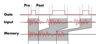
The timestamp function writes the time positions of the trigger events in an extra memory. The timestamps are relative to the start of recording, a defined zero time, externally synchronized to a radio clock, an IRIG-B a GPS receiver. Using the external synchronization gives a precise time relation for acquisitions of systems on different locations.
