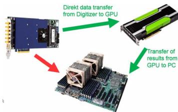
For applications requiring high powered signal and data processing Spectrum offers SCAPP (Spectrum's CUDA Access for Parallel Processing). The SCAPP SDK allows a direct link between Spectrum digitizers, AWGs or Digital Data Acquisition Cards
